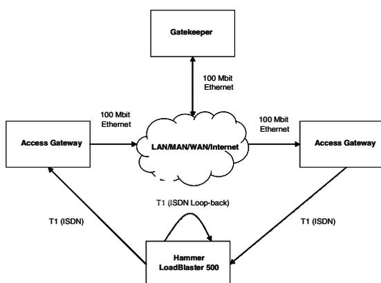
**Figure 4. Echo Example Block Diagram**
