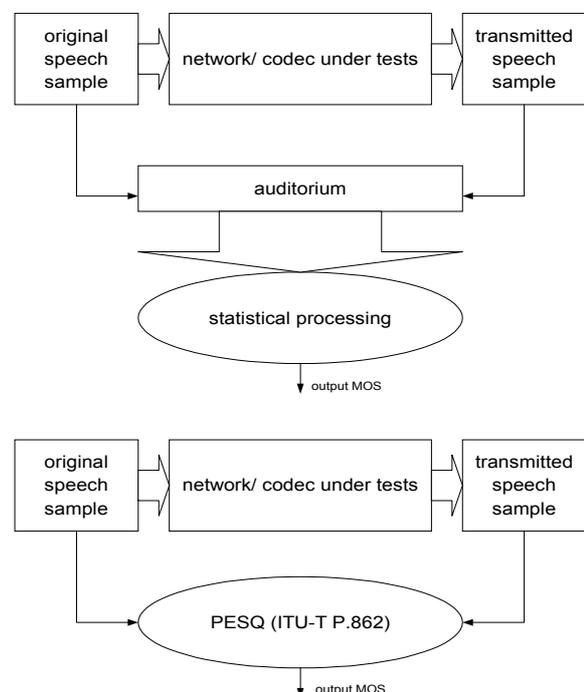
*Fig. 1. Listening tests (top) and automatic measurement of speech quality (bottom)*
