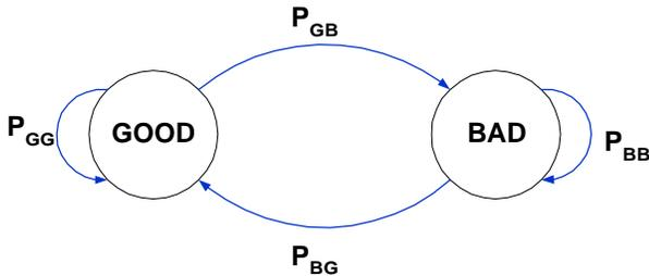
Fig. 2. 2-state Markov Delay Model
