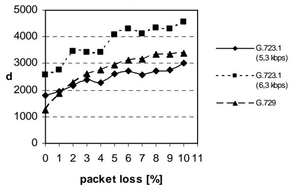
Fig.7 Graphical presentation of the simulation results of packets loss influence on the test sequence
