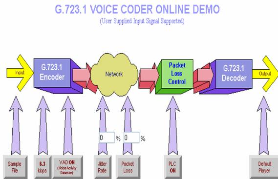
Fig.3 The simulation model of transmission chain with coder G.723.1 ITU-T
