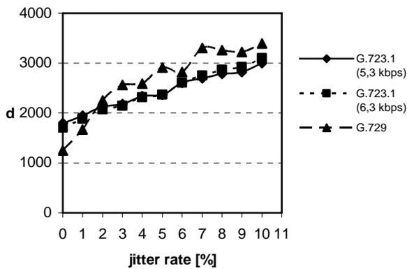
Fig.4 Graphical presentation of the simulation results of jitter influence on the test sequence
