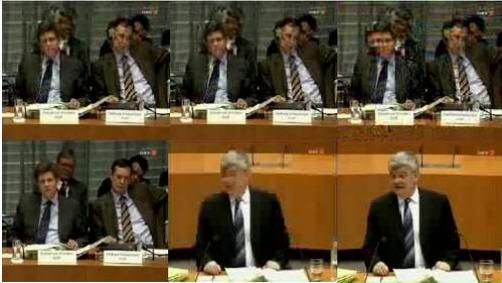
Fig. 6. Screenshots from a part of the video stream with impairments caused by packet loss (top) and without them (bottom). A frame loss causes a degradation that results in low PSNR. However, the end-user recognizes such error much later.
