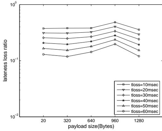
Fig. 7. Latency loss for group-2 measured data
