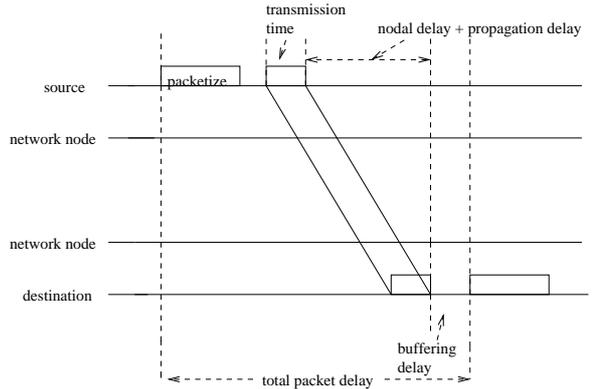
Fig. 2. Packet delay in network node
