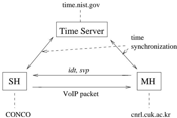
Fig. 4. Time synchronization and delay measurement
