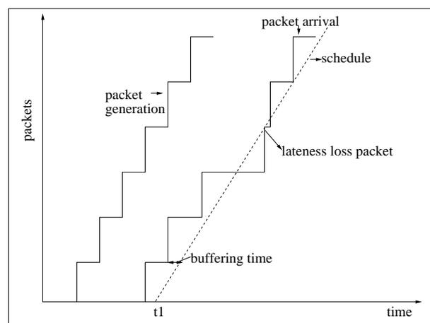
Fig. 1. Divergent goals of minimizing buffer time and minimizing late packet loss
