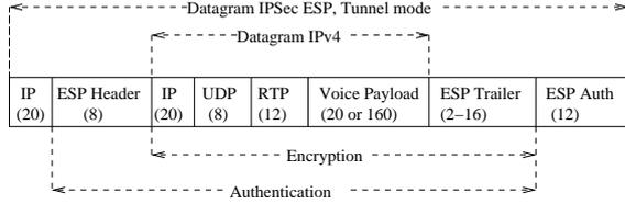
Fig. 3. IPsec ESP tunnel datagram and header size(in bytes)
