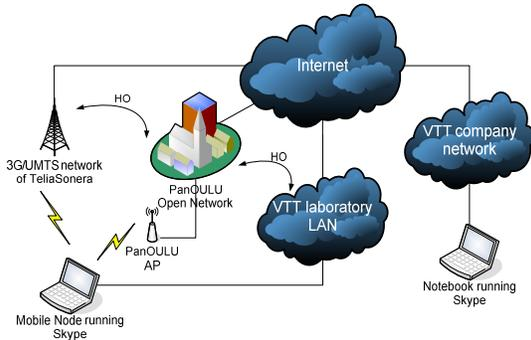
Figure 2: Experimental setup for the Mobile IP scenario. The MIP client chose the optimal connection at any given time.
