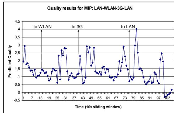
Figure 10: Quality results for the Mobile IP scenario. Three handovers were performed in this example. The quality was particularly bad, and noticeably variable during the test.
