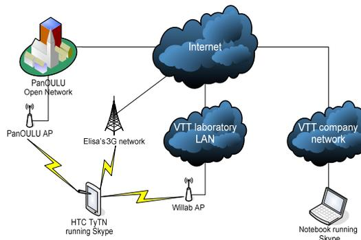
Figure 1: Experimental setup for the smartphone scenario. At any given time, the device was connected to only one of the three available networks.
