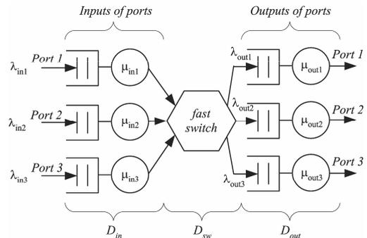
Fig. 1 Three port network node queuing model
