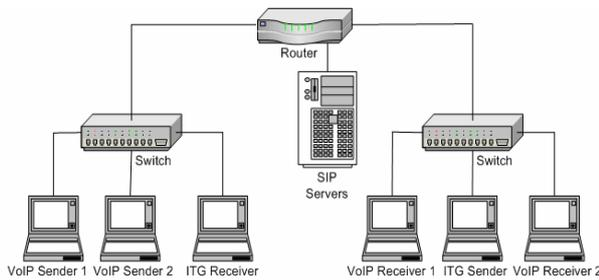
Fig.12 A typical network scenario in the environment of IP networks
