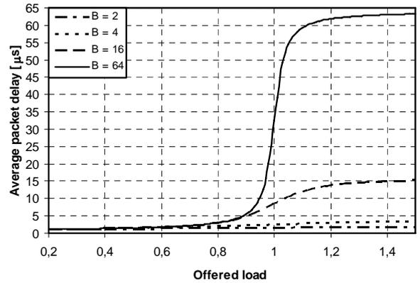
Fig. 3 Average packet delay versus offered load
