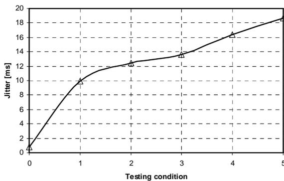
Fig.8 Impact of background traffic on average value of jitter in *VoIP* connection
