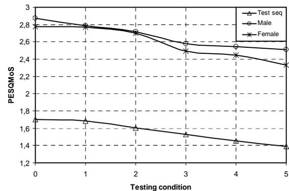
Fig.10 Impact of background traffic on speech quality of speech sequences and test sequence
