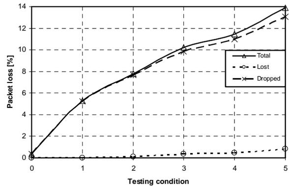
Fig.9 Impact of background traffic on packet loss in *VoIP* connection
