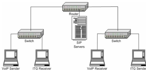
Fig.4 Measurement setup
