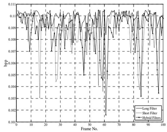
Fig. 4 Foreman QCIF video sequence Inter-Frame coded at 28kbps, 10fps, with 6 decomposition levels, with frame difference displacement predictor: (a) PSNR, and (b) bpp.
