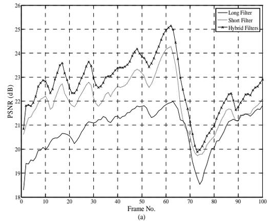
Fig. 2 Foreman QCIF video sequence Intra-Frame coded at 28kbps, 10fps, with 6 decomposition levels, with long, short, and hybrid filters: (a) PSNR and (b) bpp.
