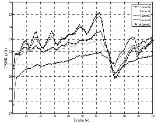
Fig. 8 The PSNR of Foreman QCIF video sequence coded at 28kbps, 10fps, with 6 decomposition levels, and different decomposition levels.
