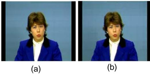
Fig. 6 Claire Frame 47, (a) Original, and (b) Decoded at 28kbps, 6 decomposition levels, with Inter-Frame hybrid filters codec, PSNR=35.19, bpp=0.038.
