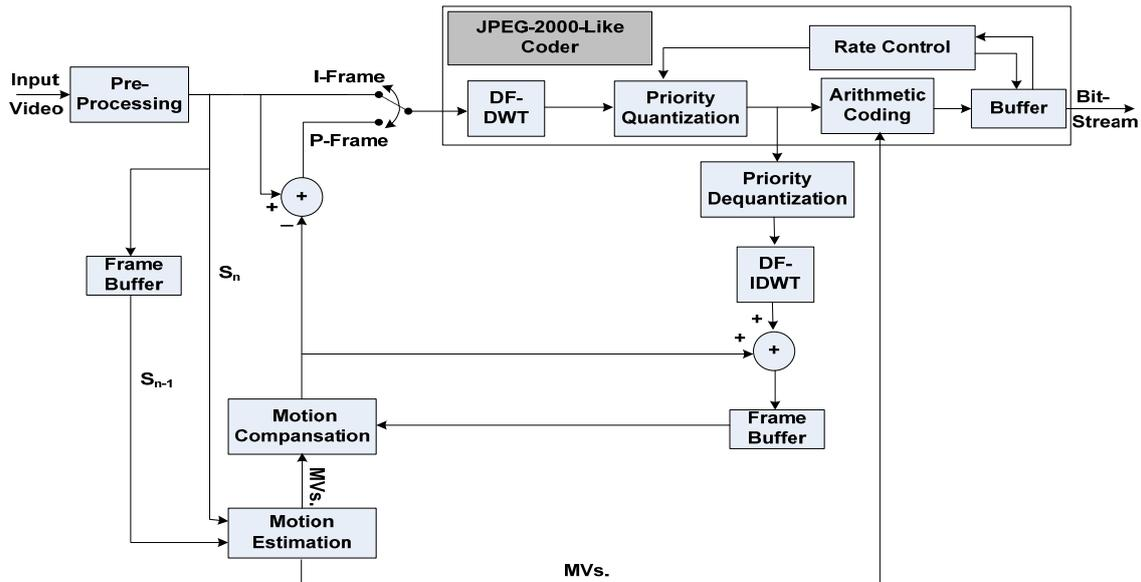
Fig. 1 Wavelet-based Video Codec
