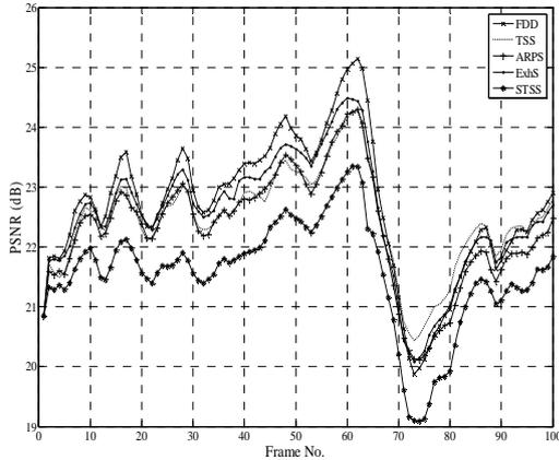
Fig. 7 The PSNR of Foreman QCIF video sequence coded at 28kbps, 10fps, with 6 decomposition levels, and different motion estimation methods.
