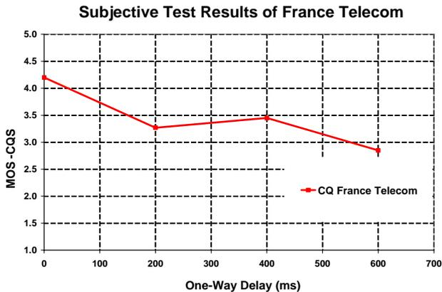
Fig. 3 Subjective test results of France Telecom experiment [4]. The results are again (like ERL -5db in Fig. 2) non-monotonic.
