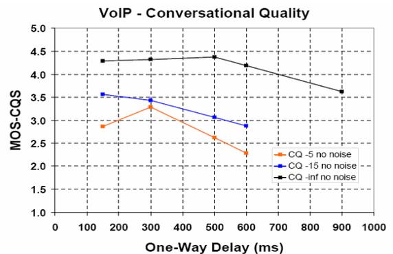
Fig. 2 Subjective test results in Czech experiment. The results for -5dB ERL are non-monotonic. Data for delay of 0 ms are not available, however, it is highly presumable all three curves converge to single value of app. 4.5 MOS.
