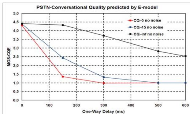
Fig. 1 E-model (G.107) output for 3 different ERL levels (-5dB, -15dB and no echo). Both cases with echo are monotonic.
