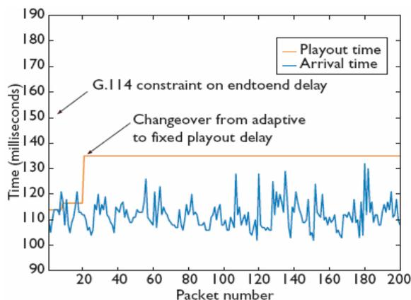
**Fig. 3:** With time synchronization, switching from an adaptive to a fixed play-out delay minimises late-arriving packet loss and silence period distortion. In this case, it results in an end-to-end delay of 135 milliseconds.
