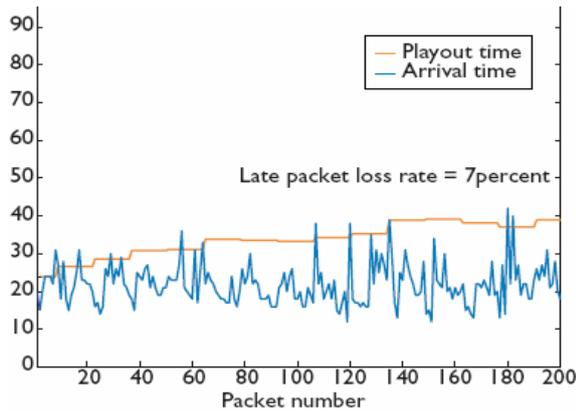
**Fig. 2:** Adaptive buffer performance. The y-axis scale illustrates the inter-packet arrival-time variance (jitter) resulting principally from variable queuing delays. The dark line indicates the play-out time of each packet relative to its arrival time.
