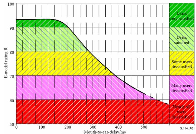
**Fig. 4:** G.114 – Determination of the effects of absolute delay by the E-model [11]
