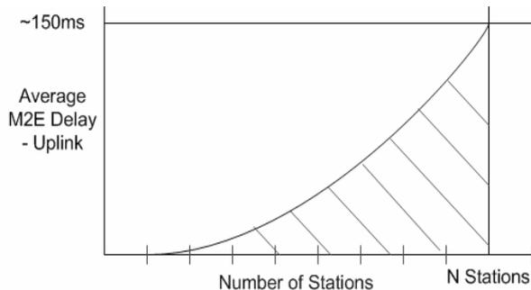
**Fig. 5:** Average uplink delay; MAC delay + Other delays = M2E delay
